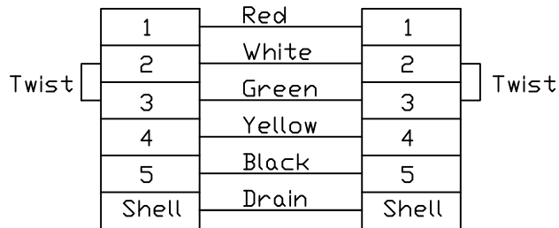
Micro USB-B Plug Conn. Wiring Diagram
